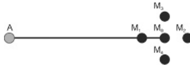
Figure 3 Scheme of the current and measuring electrode distribution for the tensor array, TEN FD .
