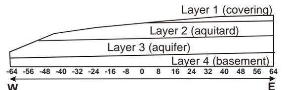
Figure 6: Structural section for the study area.
