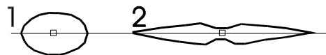
Fig.1. Comparison of ARS diagram for linear (1) and non-linear (2) arrays over anisotropic halfspace with \lambda=1.73
